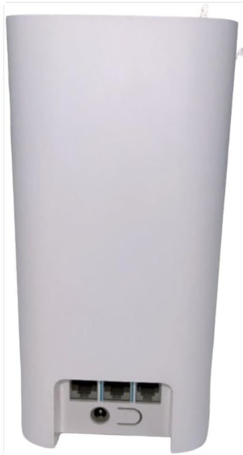
Figure 4.1: Back view of the STC 5G CPE 5 Router H155-383. This image shows the multiple LAN/Ethernet ports, the power input, and a reset button.
