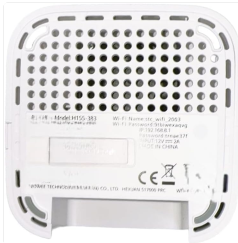
Figure 3.1: Bottom view of the STC 5G CPE 5 Router H155-383. This image displays the ventilation holes, product label with model number and default Wi-Fi credentials, and the SIM card slot.
