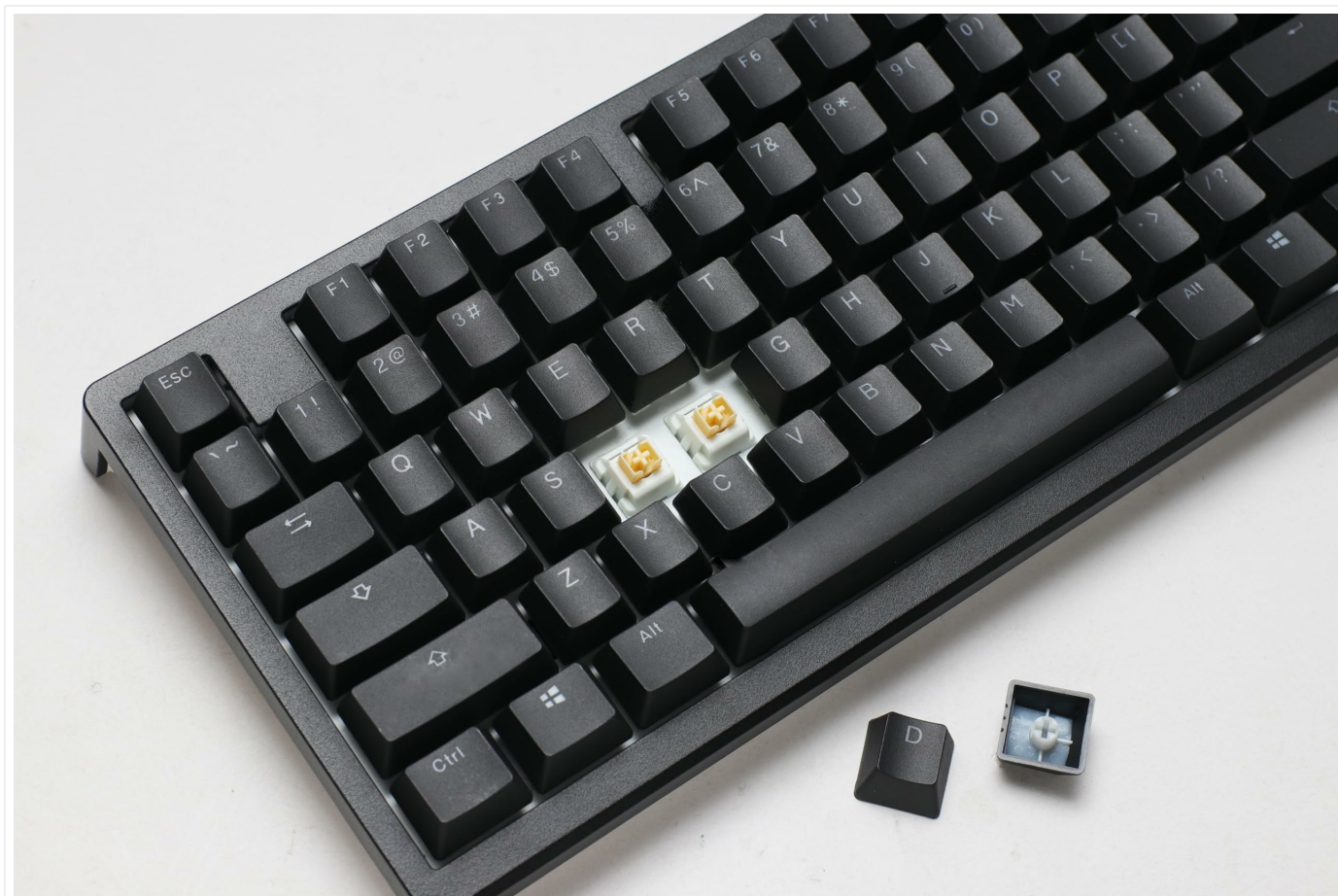
Image: A close-up view of the keyboard with two keycaps and their underlying Cherry MX2A Blue switches removed, revealing the hot-swappable sockets beneath. This demonstrates the ease of switch replacement.
