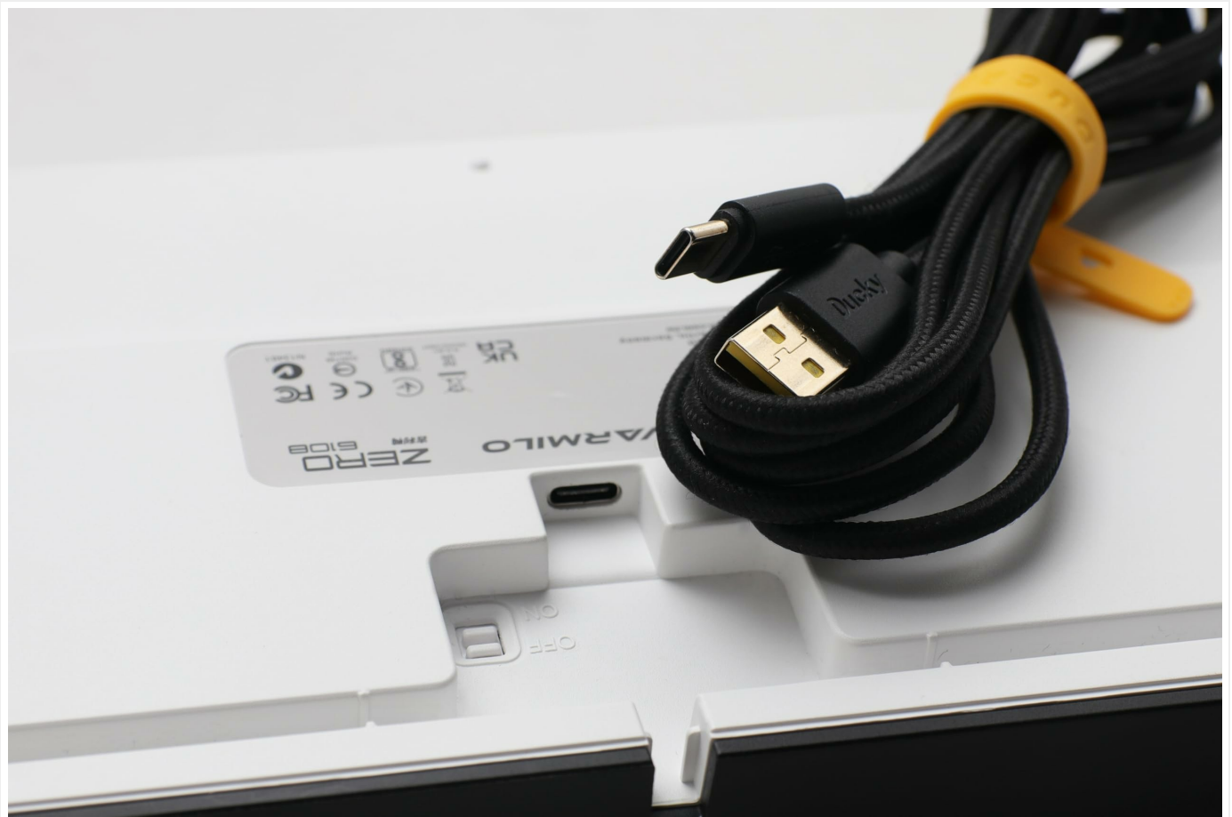
Image: The USB-C port located on the back of the keyboard, with the braided USB-C to USB-A cable connected. This port is used for wired connection and charging.
