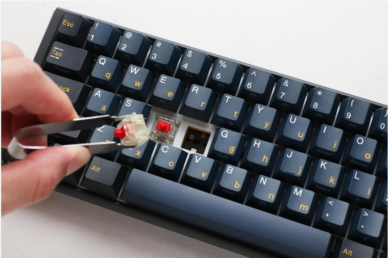
Image 5.1: A hand demonstrating the use of a switch puller to safely remove a mechanical switch from the keyboard's hotswap socket.
