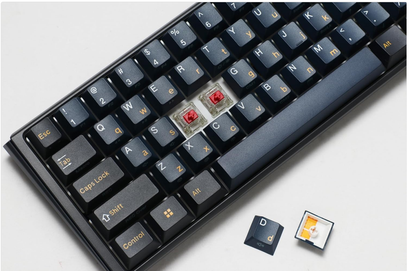
Image 5.2: A close-up view of the keyboard with several keycaps and switches removed, revealing the hotswap sockets and the internal structure.
