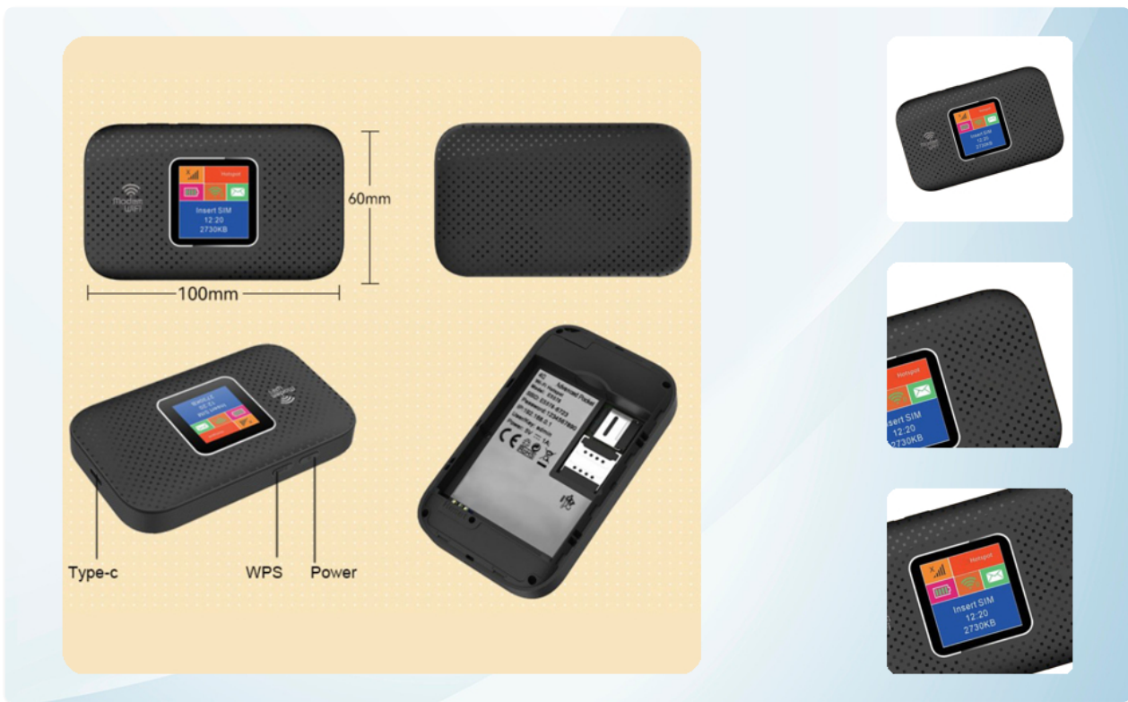
Image 1.1: The ASHATA Portable Pocket WiFi Router, highlighting its compact design, Type-C interface, and 3000mAh battery capacity.
