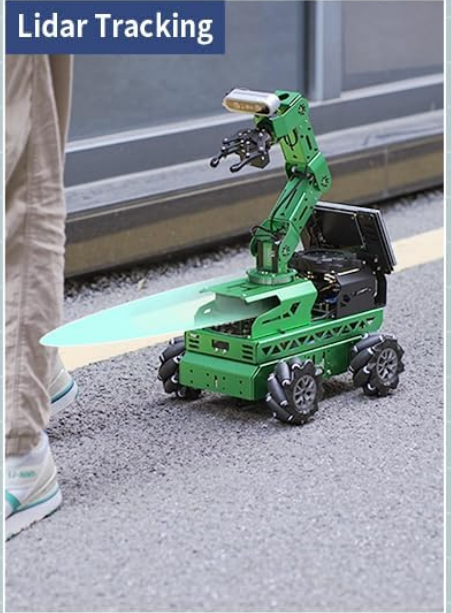
Figure 5.1: Lidar functions including mapping (Cartographer, Hector, Karto, Gmapping), voice navigation, obstacle avoidance, multi-vehicle navigation, and Lidar tracking.
