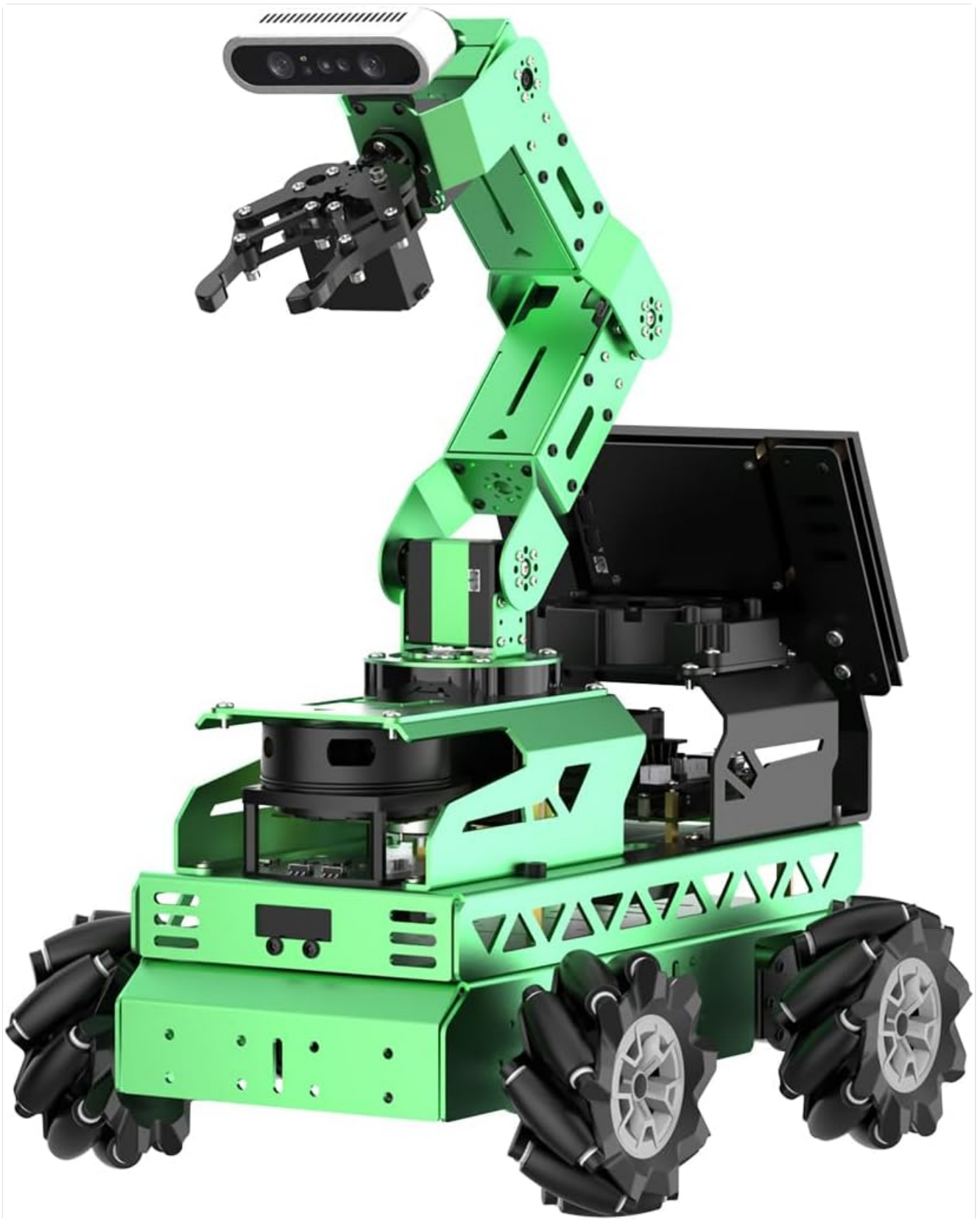
Figure 2.1: HIWONDER JetRover Robot Car with 6DOF Robotic Arm and various sensors.
