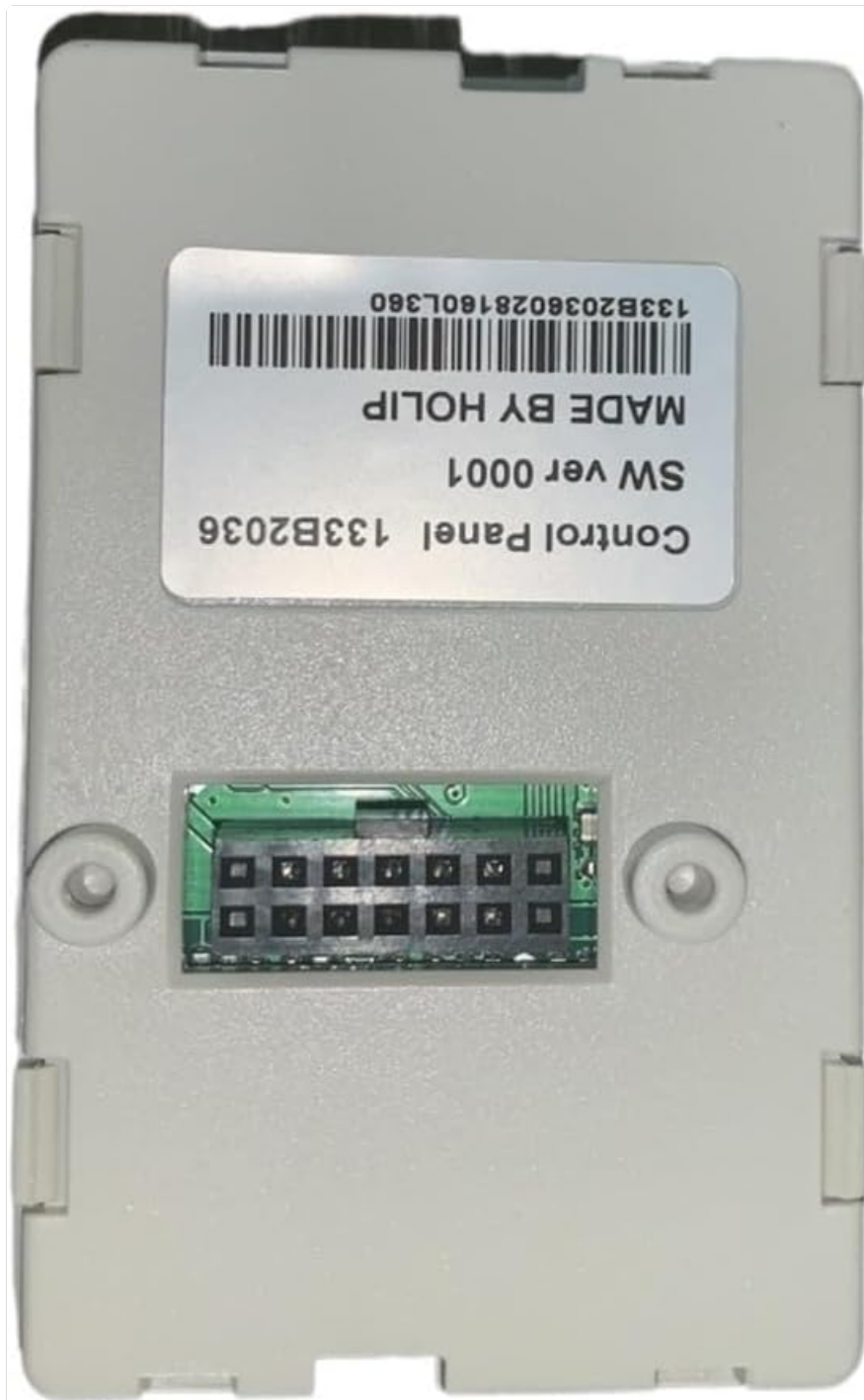
Figure 2: Rear view of the Inverter Panel. This image displays the back of the control panel, featuring a label with model information and a barcode. A multi-pin connector is visible, which is used for connecting the panel to the inverter system.
