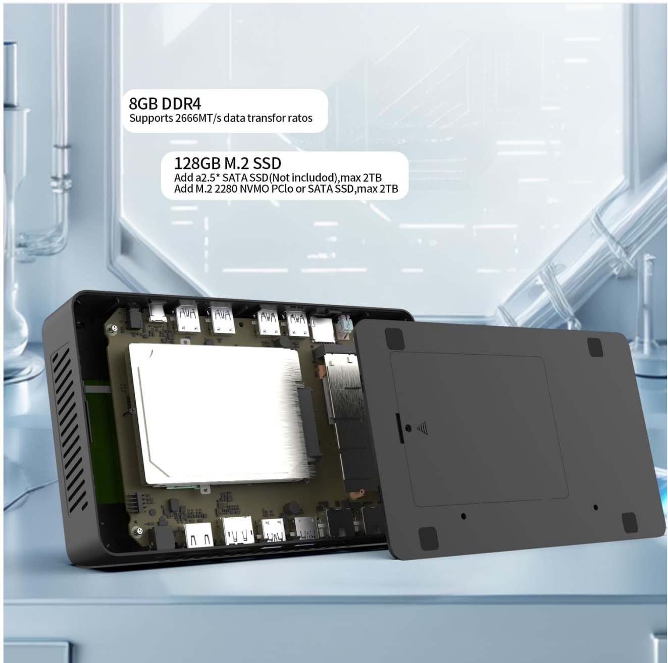
Figure 5.1.1: Internal Components and Storage Expansion. This image provides an internal view of the EVRAIN T8 PRO Mini PC, highlighting the 8GB DDR4 RAM and the 128GB M.2 SSD. It also shows the accessible compartment for adding a 2.5-inch SATA SSD (up to 2TB) or an M.2 2280 NVMe PCIe or SATA SSD (up to 2TB).
