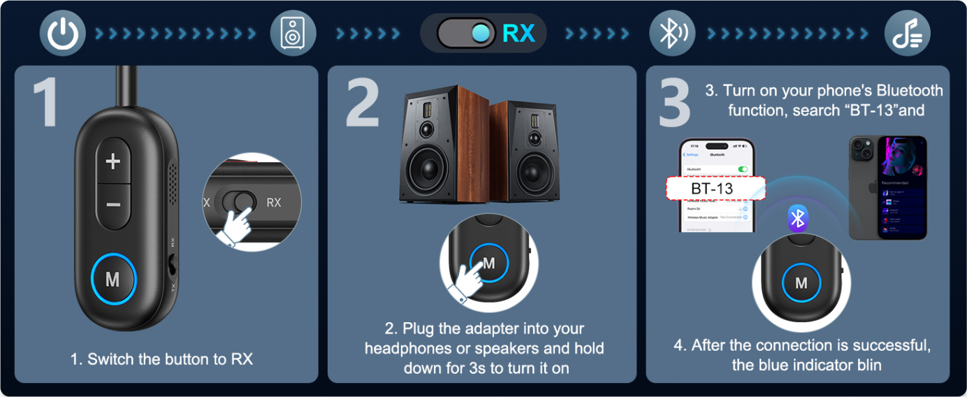
Image: A visual guide demonstrating the steps for connecting the Ankilo adapter in RX mode, showing the switch, plugging into speakers, and pairing with a smartphone.
