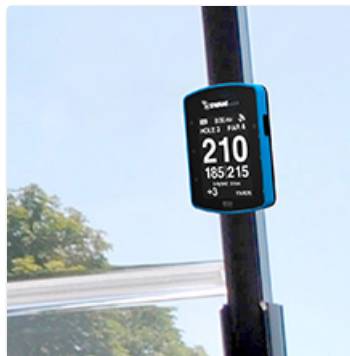
Figure 3: The Swami KISS 2.0 securely attached to a metal surface on a golf cart using its integrated magnets.
