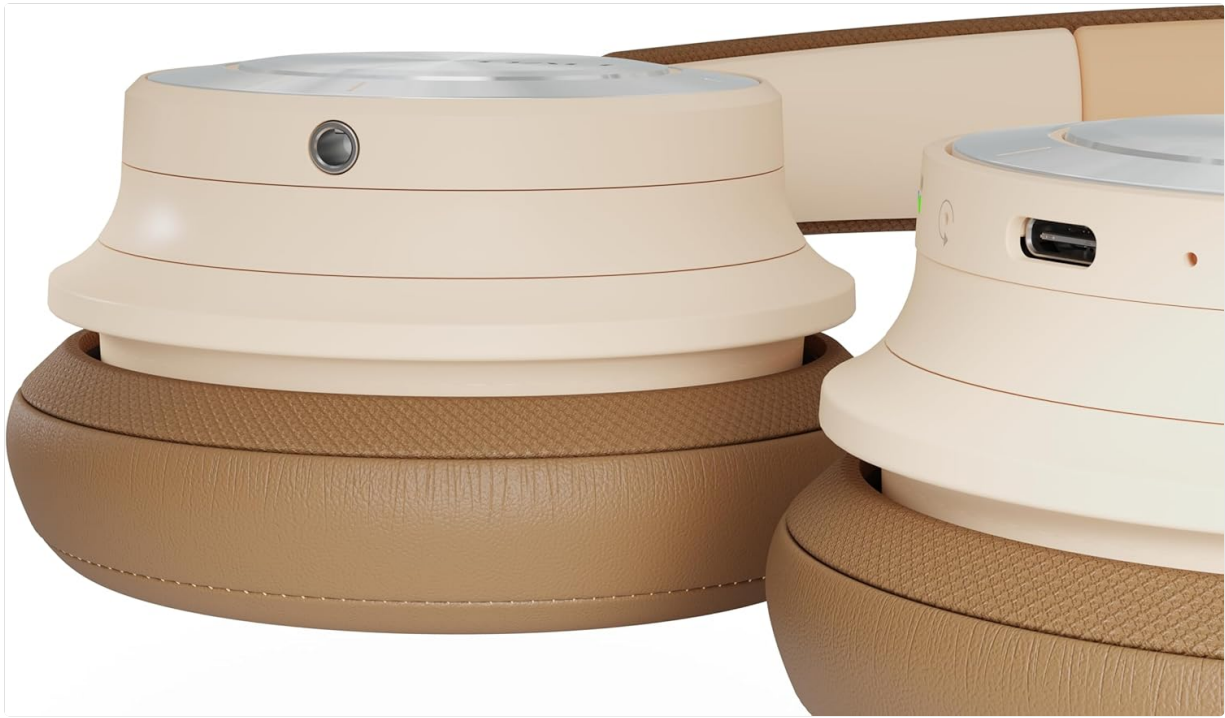
Figure 2.4: Close-up view of the DALI IO-8 earcup, showing the USB-C charging port and other control buttons.
