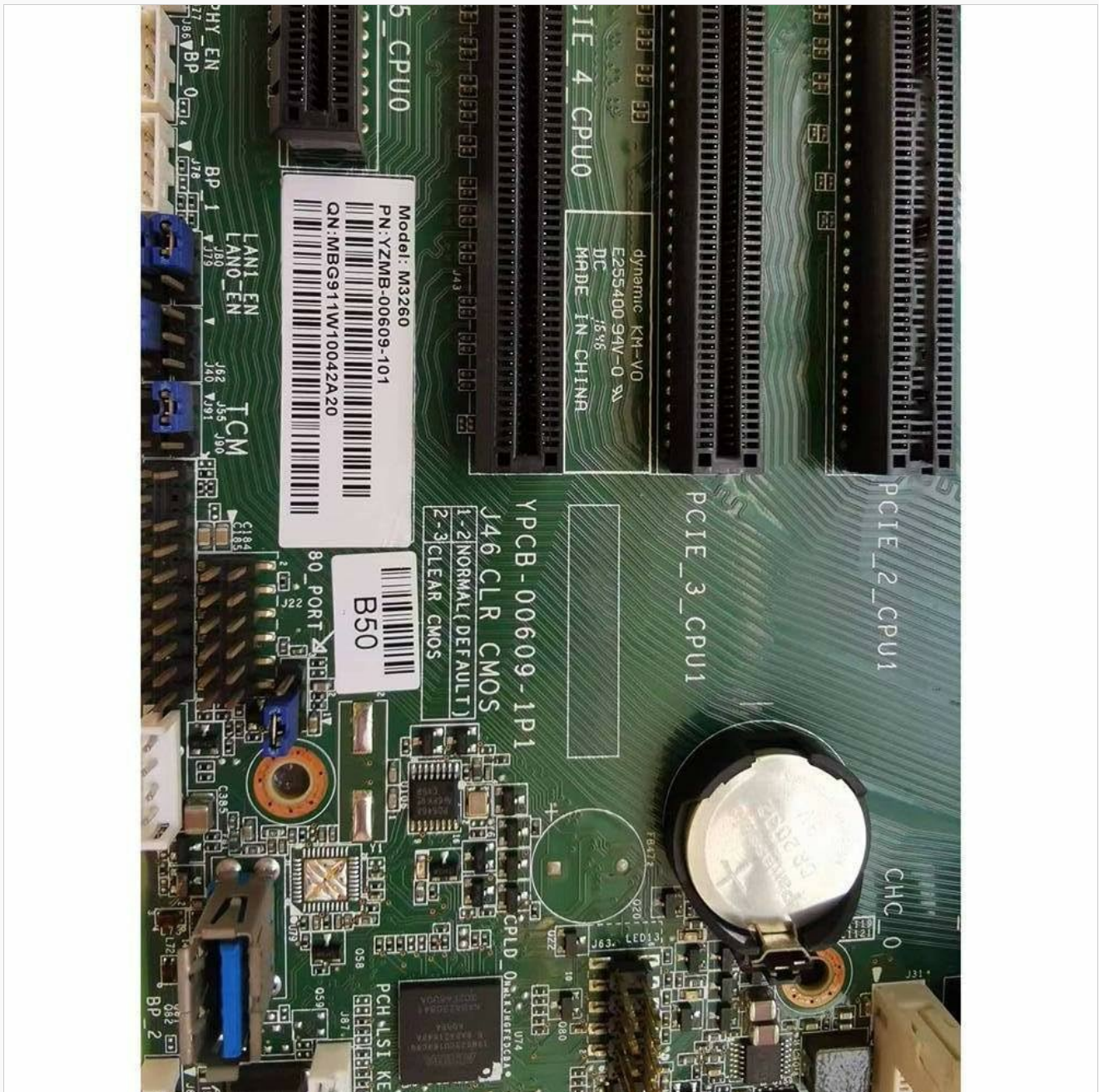
Figure 1: M3260 Motherboard Component Detail. This image provides a detailed view of the motherboard's central area, highlighting the CPU socket, multiple RAM (DIMM) slots, and PCIe expansion slots. Key labels visible include the model number M3260, part numbers YZMB-00609-101 and YPCB-00609-1P1, and a CMOS clear jumper labeled J46. CLR CMOS. Other connectors such as LAN_EN, TCM, and 80 PORT are also visible, along with the CMOS battery (B50).
