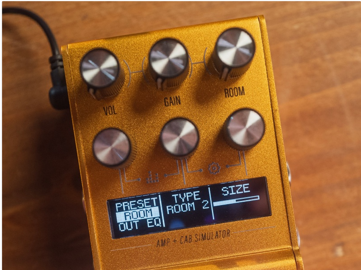
Figure 5: Room Settings Display. This image shows the ACS1 display indicating the "ROOM" parameter, with "TYPE ROOM 2" and "SIZE" visible, allowing users to adjust the simulated room acoustics.
