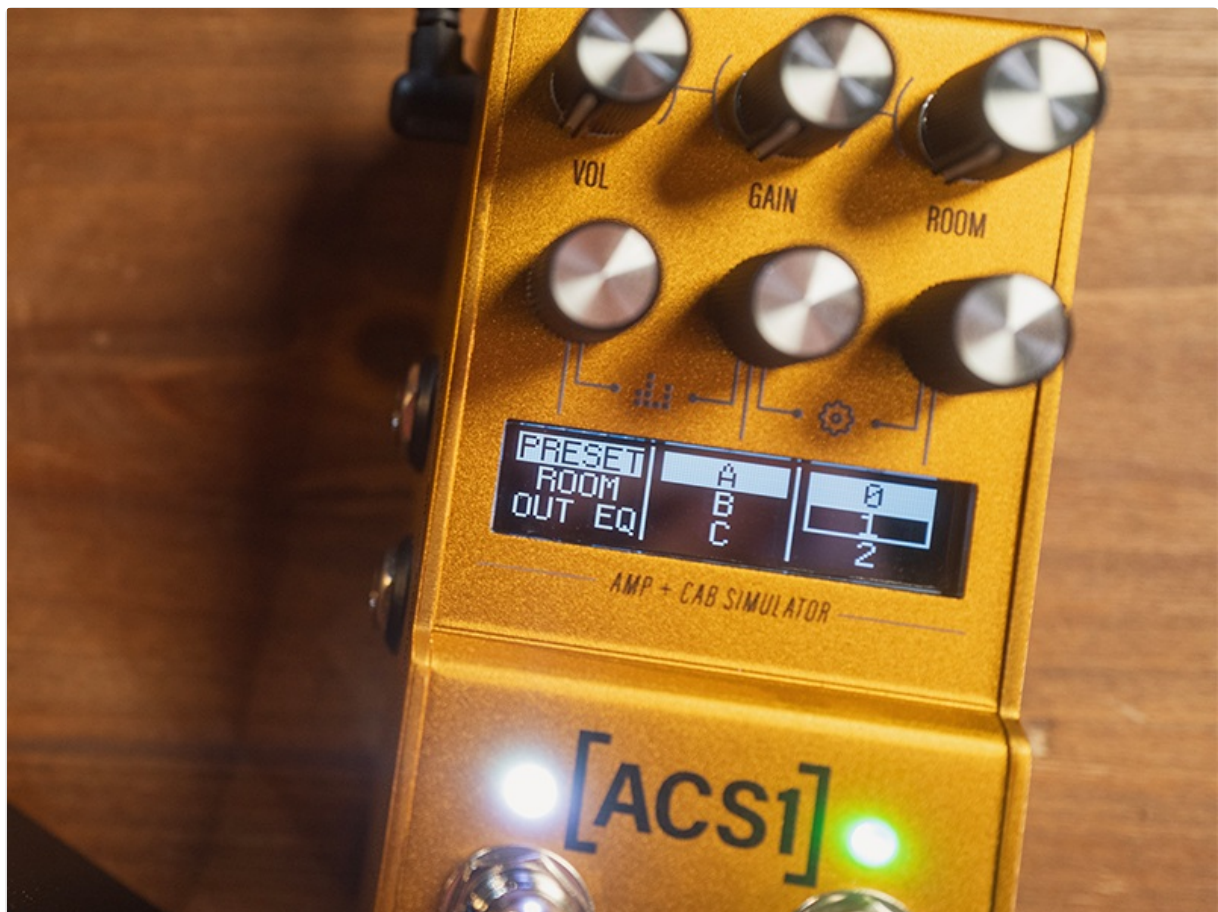
Figure 6: Preset Selection Interface. This display shows the "PRESET" menu, with options for selecting different preset slots (A, B, C) and their corresponding numbers (0, 2).
