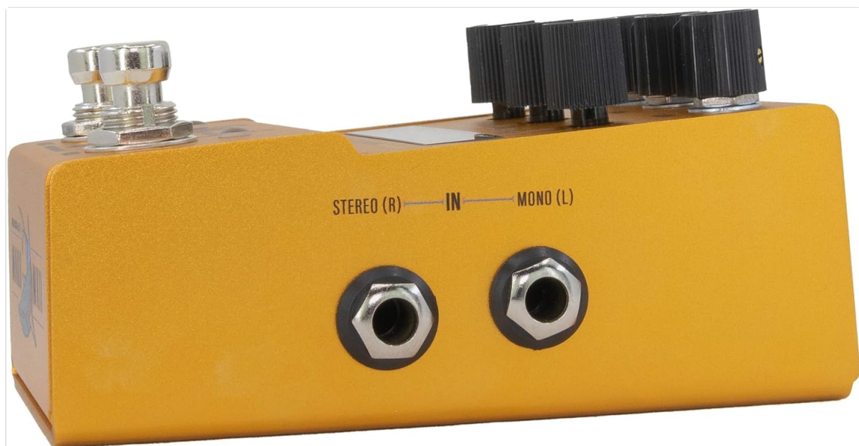
Figure 2: Input Side View. This image shows the right side of the pedal, featuring the Mono (L) and Stereo (R) input jacks. These are used to connect your instrument or other pedals to the ACS1.
