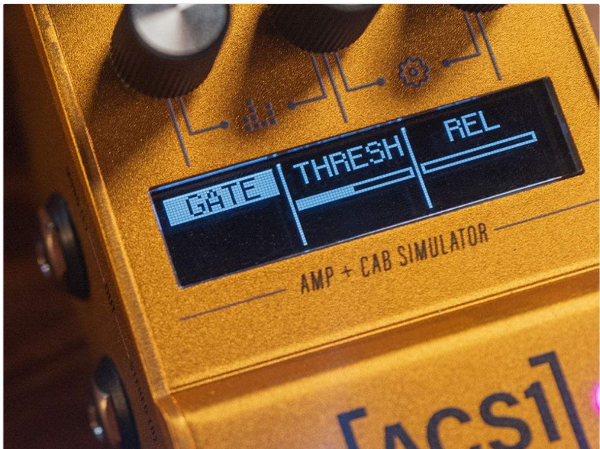
Figure 7: Noise Gate Settings. This image shows the ACS1 display with the "GATE" menu active, allowing adjustment of "THRESH" (Threshold) and "REL" (Release) parameters for noise reduction.
