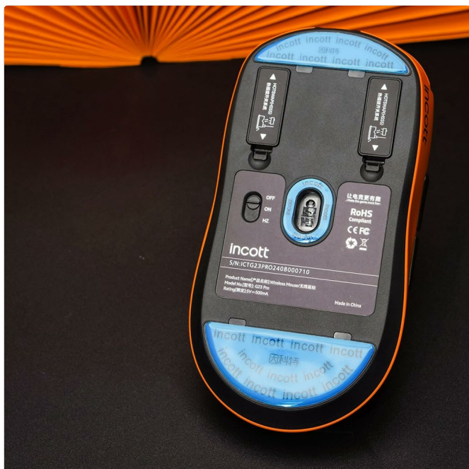
Image: Bottom view of the Incott G23 Series Gaming Mouse, showing the sensor, power switch, and hot-swappable switch compartments.
