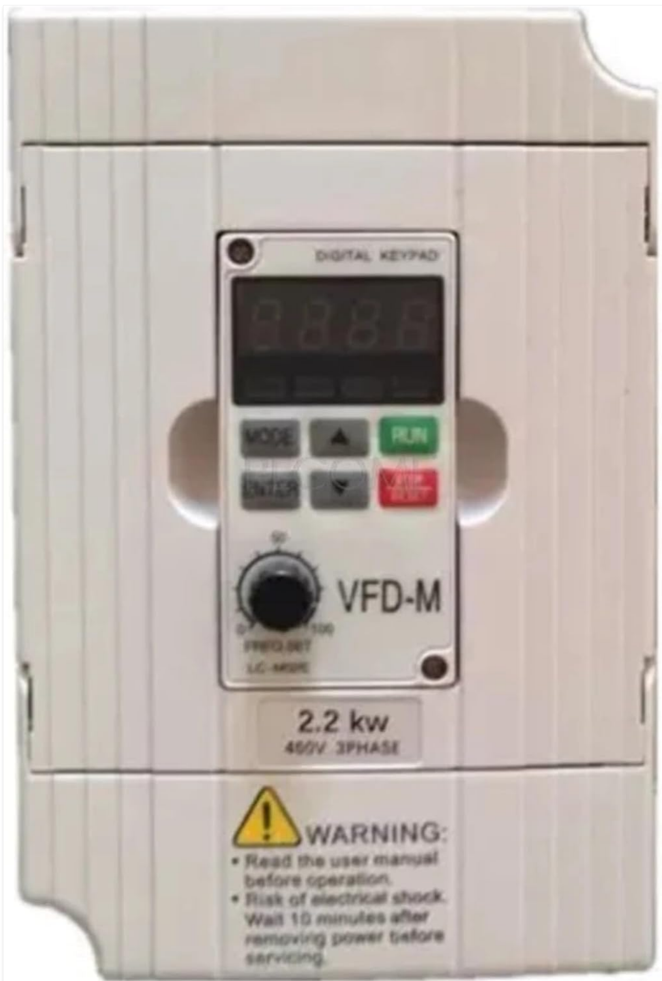
Figure 1.1: Front panel of the VFD-M Series Frequency Inverter, showing the digital display, control buttons (MODE, RUN, ENTER, STOP/RESET), and a rotary frequency adjustment knob. A warning label is visible at the bottom.
