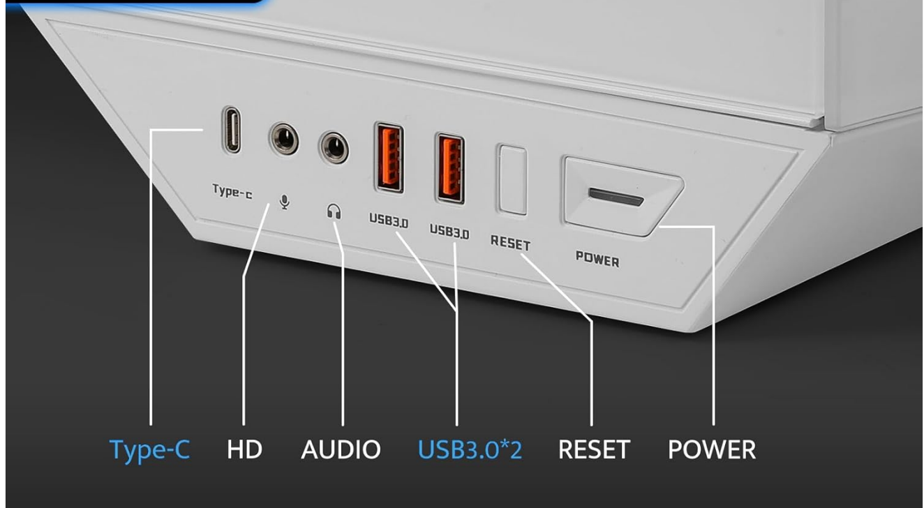
Image 4.6: Detailed view of the front I/O panel.
