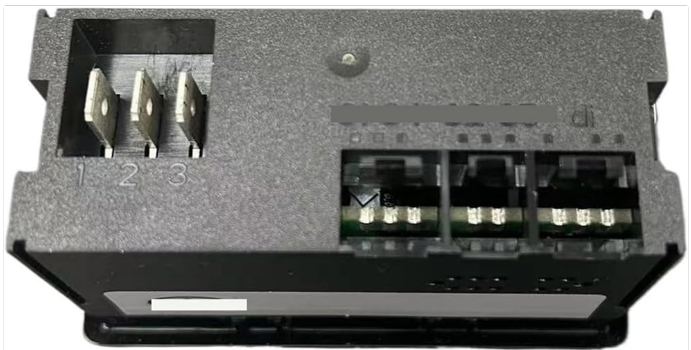
Figure 3.2: Rear view of the Bolisila ERC111A Temperature Controller. This image displays the wiring terminals for power input, digital
