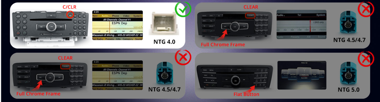
Figure 2.1: Benz COMAND NTG Identification. Ensure your vehicle has the NTG 4.0 system for compatibility.
