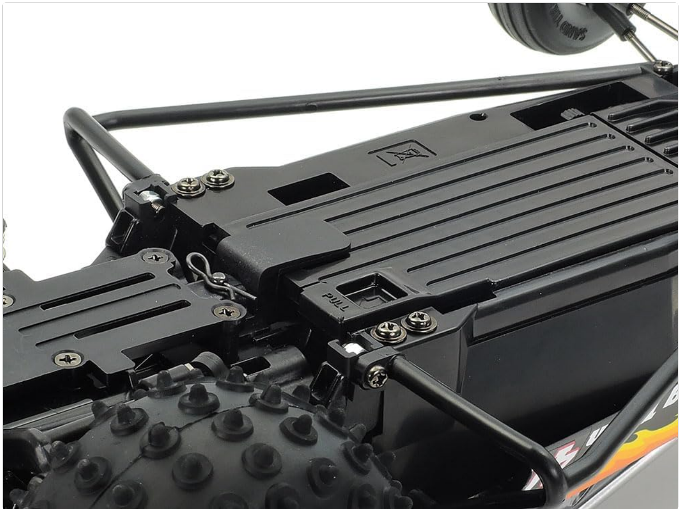
Figure 4.1: Battery compartment with securing mechanism.
