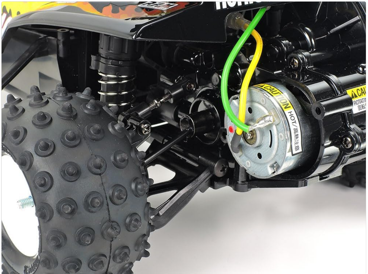
Figure 3.3: Detail of the rear motor and DT-02 based transmission.
