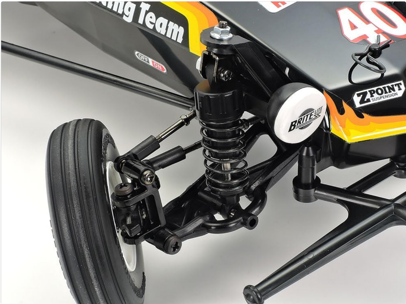
Figure 3.2: Detail of the front independent suspension.
