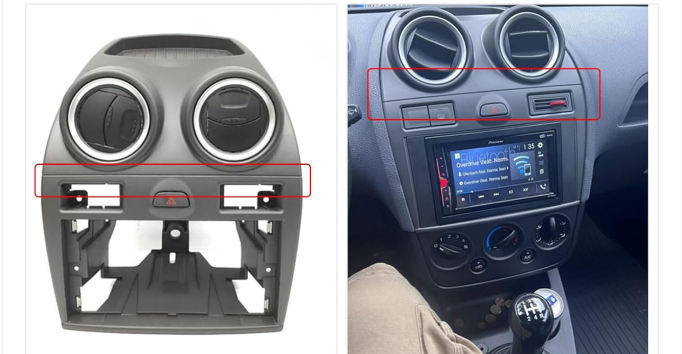
Image 5.1: Visual guide for checking the compatibility of your Ford Fiesta Mk5 center console. The image illustrates the difference between a split and an unsplit console frame.
