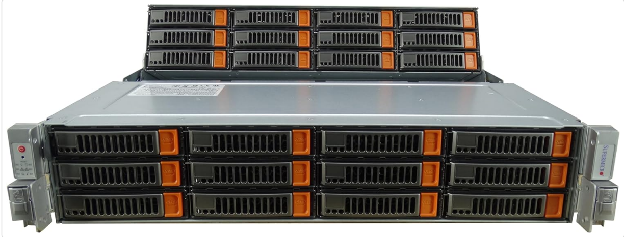
Figure 3.3.1: Front view of the Supermicro 6028R-E1CR24N server, showcasing its 24 Large Form Factor (LFF) drive bays. Each bay is designed to accommodate a 3.5-inch hard drive or SSD, providing substantial storage capacity. The server also features two flex bays, visible on the right side, which can be used for additional storage or other modules.
