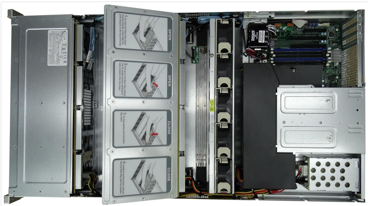
Figure 3.3.2: Top-down internal view of the Supermicro 6028R-E1CR24N server. This image provides a clear look at the internal layout, including the motherboard, CPU heatsinks, RAM slots, and the drive bay backplane. Instructions for opening and closing the drive bays are printed on the top cover, indicating a user-friendly design for drive installation and removal.
