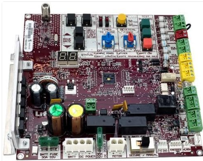
Figure 1: LiftMaster K1D8389-1CC Control Board. This image displays the main control board with various components, including fuses, capacitors, relays, and terminal blocks for connections. Key areas visible include the status display, test buttons, and adjustment potentiometers for timer and force settings.
