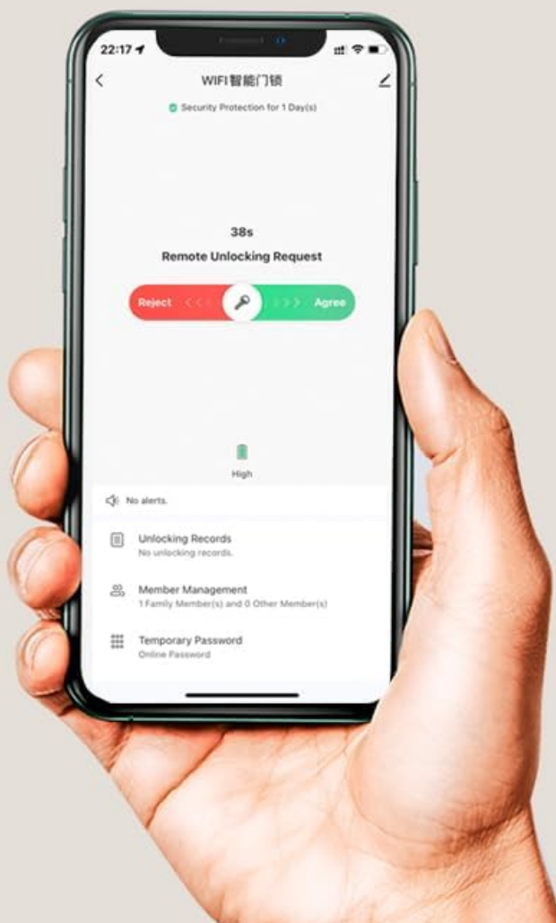
Image 5.4: Screenshot of the Tuya Smart APP interface, illustrating features such as remote unlocking requests, unlocking records, member management, and temporary password generation.
