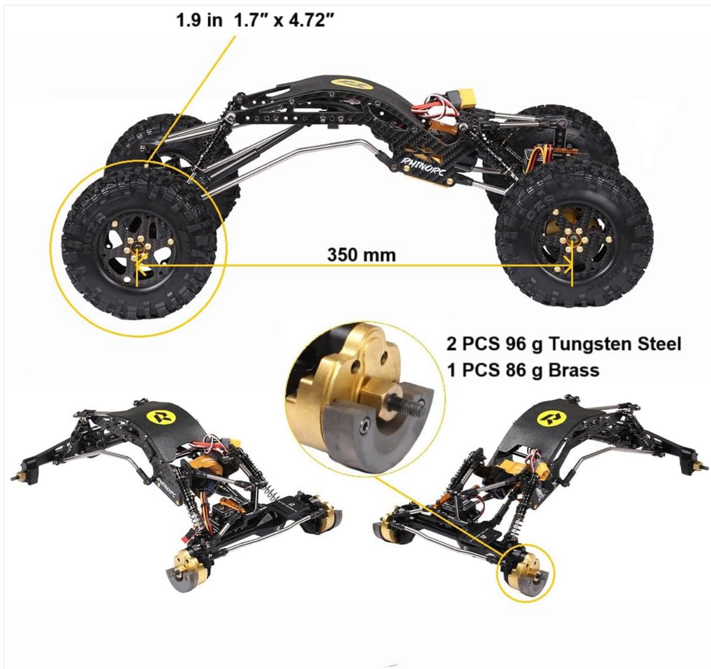
Figure 5: Close-up view of the YUE ONE V2's wheels and chassis, highlighting the 1.9-inch tire size, 350mm wheelbase, and the inclusion of 96g tungsten steel and 86g brass weights for optimal crawling performance.
