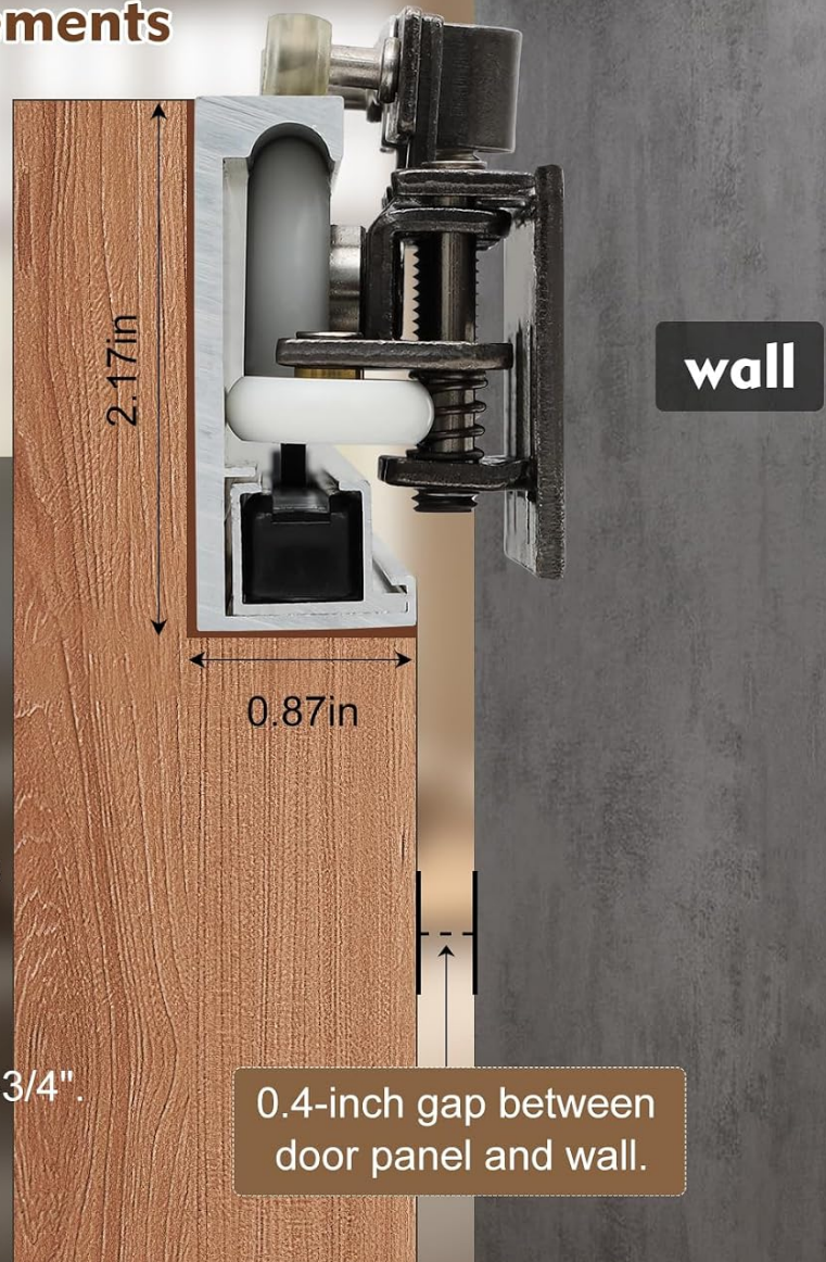
Image: Detailed diagram illustrating the required door thickness (1-1/4" to 1-3/4") and the recommended 0.4-inch gap between the door panel and the wall for proper soft-close mechanism function.
