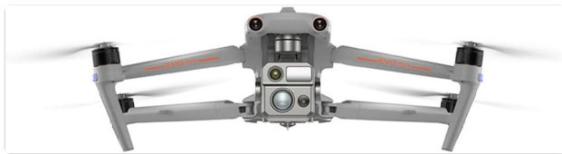
Image: Front view of the EVO MAX 4N, showing the camera and obstacle avoidance sensors.
