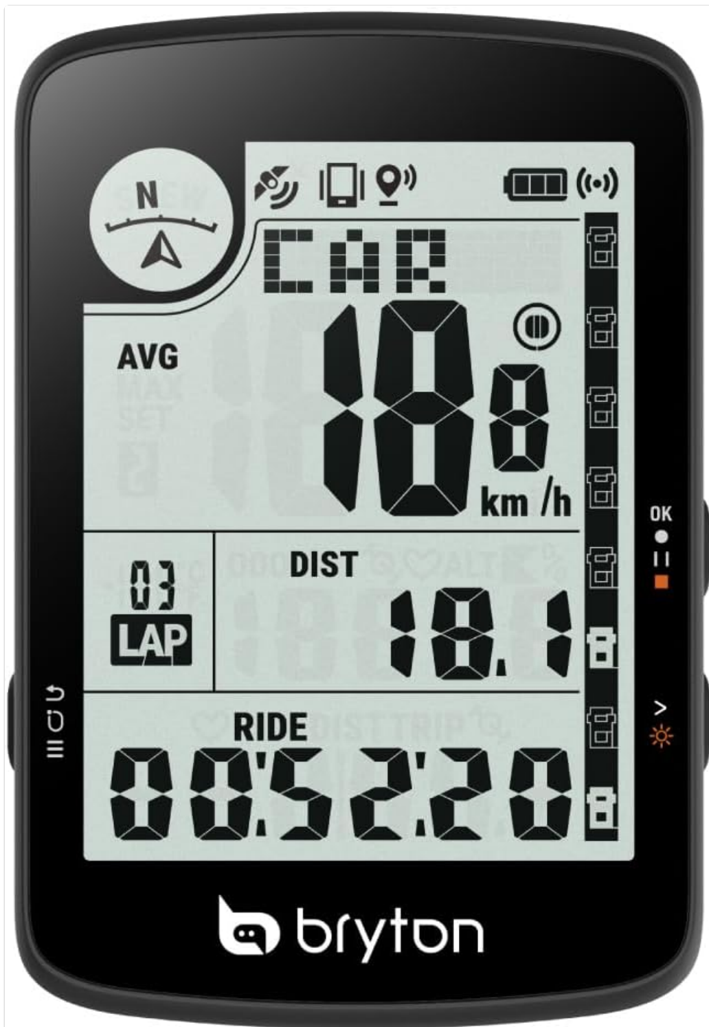
Image: A close-up of the Bryton Rider 17's LCD screen showing various data fields like speed, distance, and ride time.
