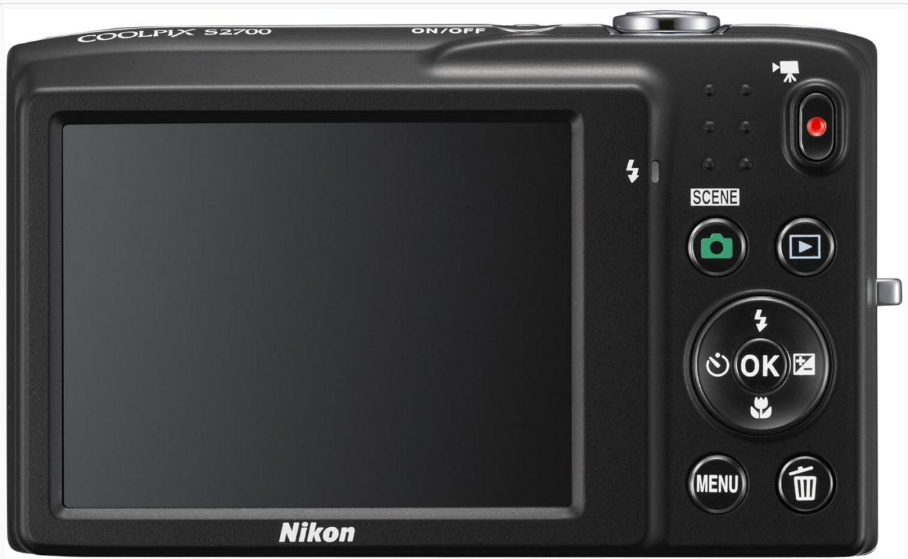
Figure 2.2: Rear View. This image shows the back of the camera, featuring the LCD screen, directional pad with 'OK' button, 'MENU' button, 'DELETE' button, 'SCENE' button, and video record button.
