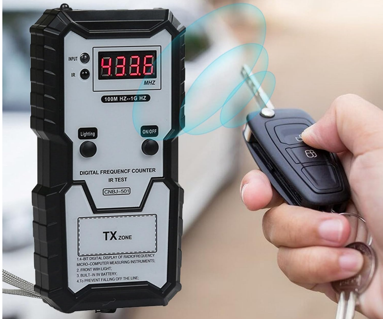
Figure 4: The tester can also detect infrared signals, indicated by the IR LED.
