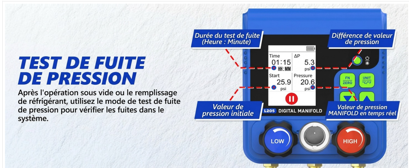
Figure 5.5: Pressure leak test display showing duration, pressure difference, initial pressure, and real-time pressure.
