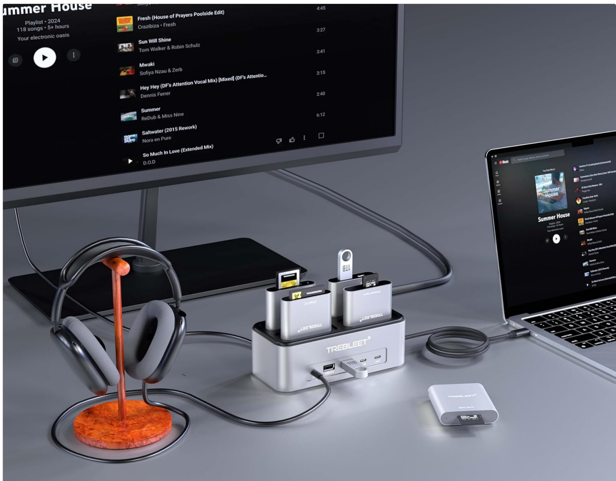
Figure 5: A typical setup showing the docking station connected to a laptop, powering and extending its display to multiple external monitors, and connecting various peripherals.
