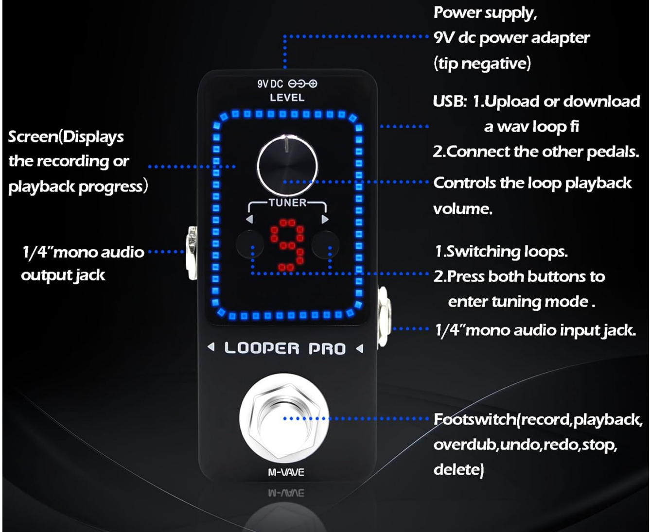
Figure 3: Diagram of the Loop Pedal Pro's control panel, highlighting input/output jacks, level knob, and buttons.
