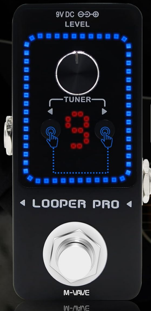
Figure 5: Visual representation of the tuner function, showing how to activate it and interpret the LED pitch indicators.
