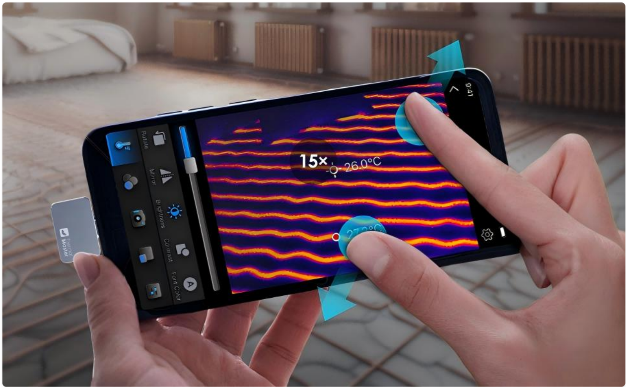
Figure 7: Demonstrating the 15x zoom feature on the P2 Pro app.
