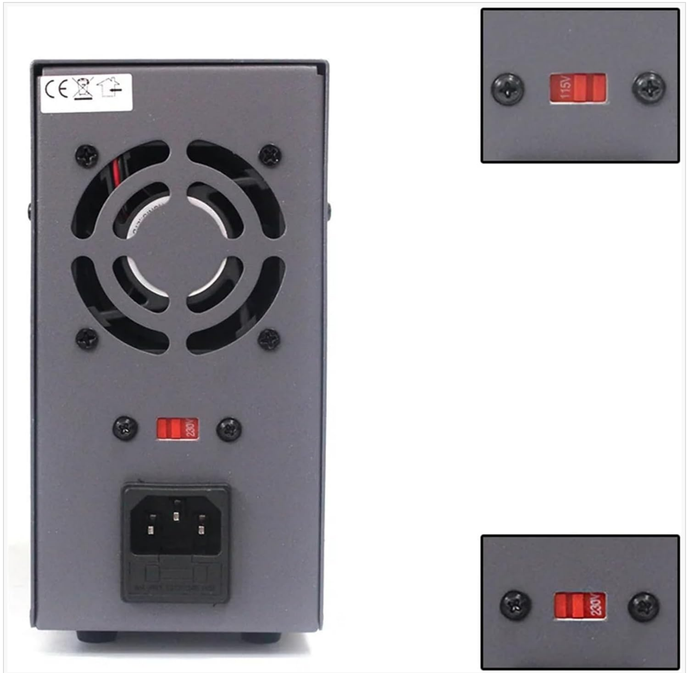
Figure 3.2: Rear view of the Aoleaby KPS605D DC Power Supply. This image highlights the AC power input socket, the fuse holder, the cooling fan, and the crucial 115V/230V voltage selector switch. Insets show the selector switch set to 115V and 230V.
