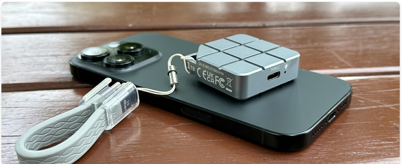
Figure 7: The MAIWO Portable SSD's aluminum alloy construction is designed for fast heat dissipation.
