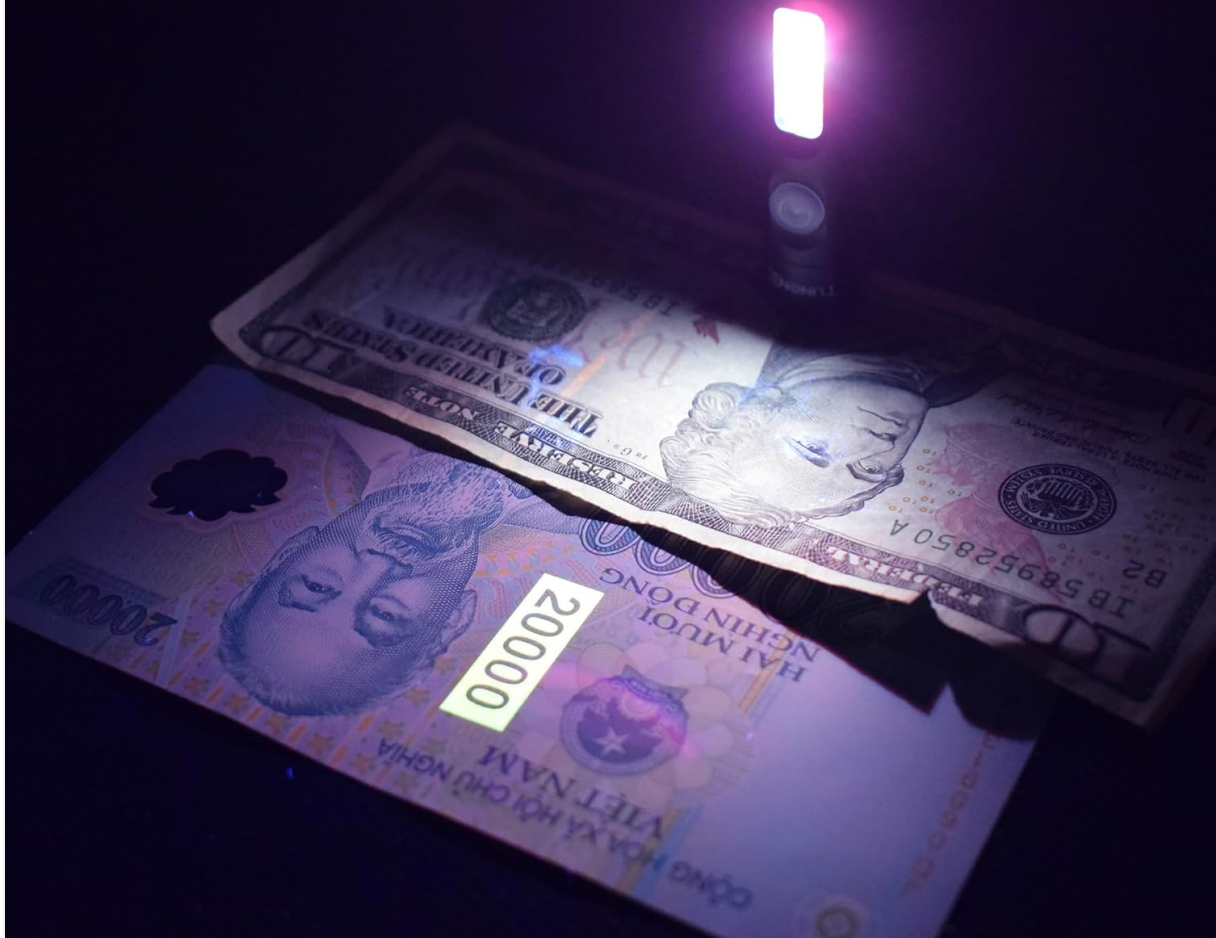
Figure 8: Using the 365nm UV light to detect fluorescent markings on currency.
