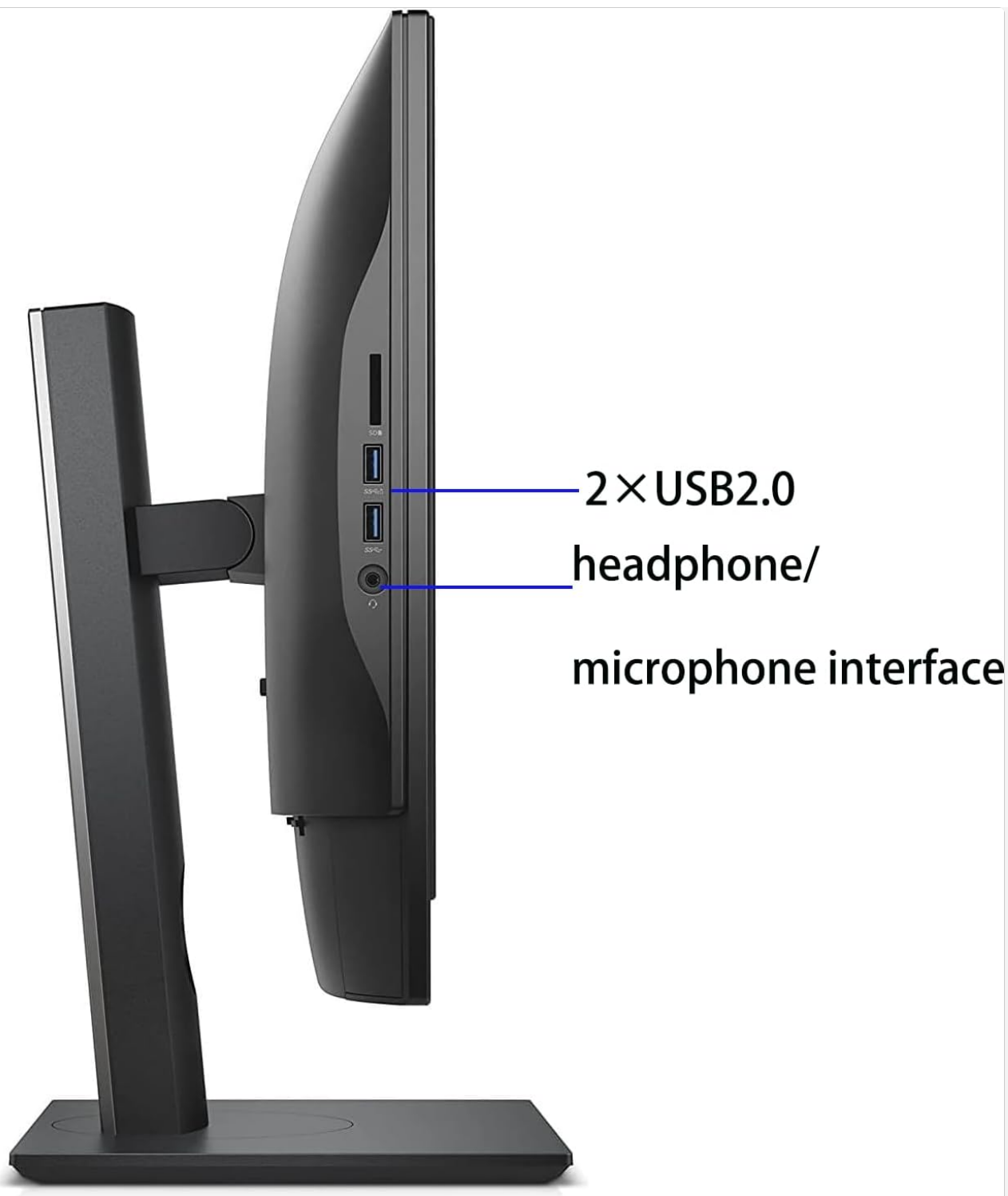
Image: Close-up of the left side of the Dell OptiPlex 5250, showing two USB 2.0 ports and a combined headphone/microphone interface.
