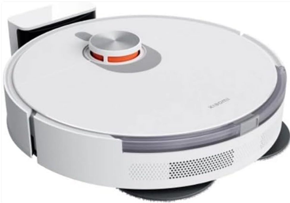
Figure 4.2: Side view of the Xiaomi Robot Vacuum S20+, illustrating the dual rotating mop pads and the side brush for edge cleaning.
