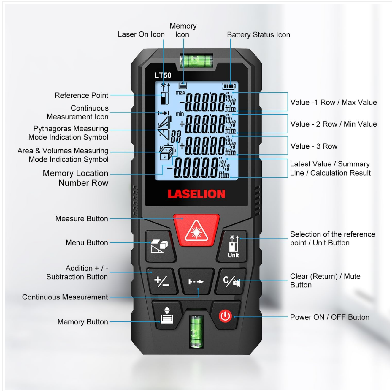
Image: Diagram illustrating the LASELION LT50's display icons and button functions, including Measure, Menu, Addition/Subtraction, Continuous Measurement, Memory, Unit, Clear/Mute, and Power ON/OFF.
