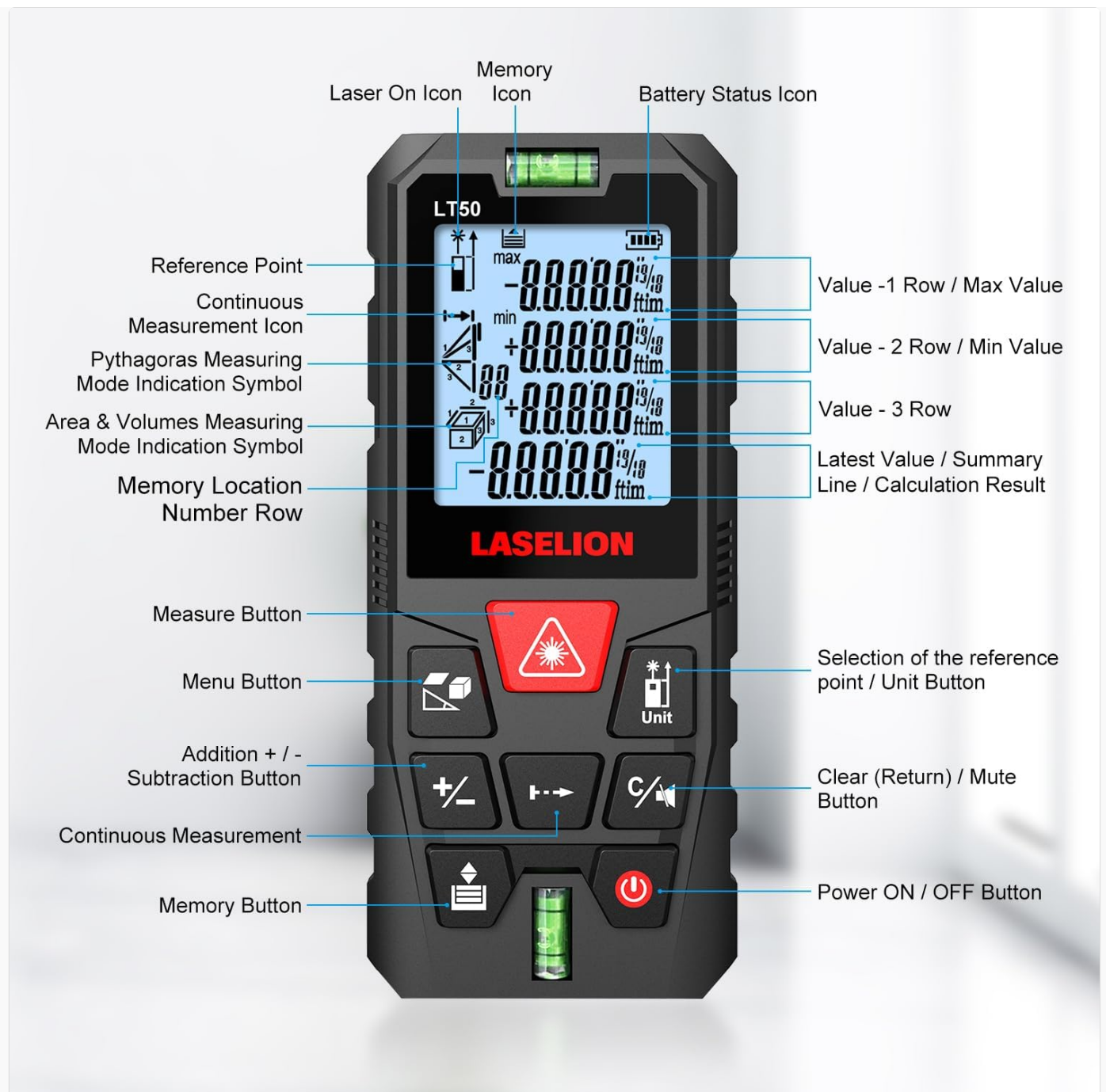
Figure 3: Detailed overview of the LT50's display and button functions.
