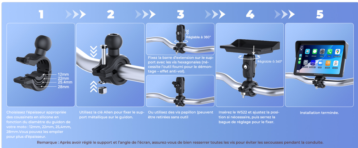
Figure 3: Detailed steps for mounting the display.
