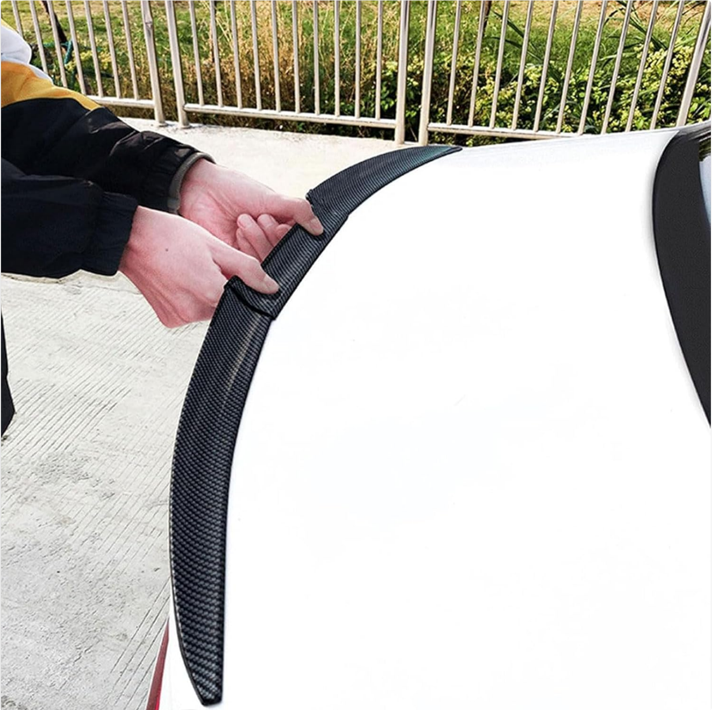
Image: A person's hands carefully pressing the carbon fiber spoiler onto the trunk lid of a white car during installation.
