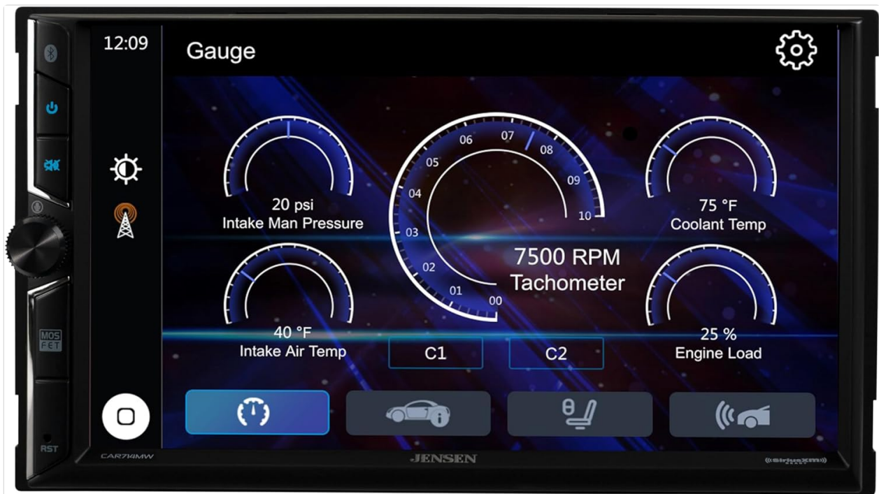
Figure 4.1: Example of the CAR714MW's gauge display interface.
