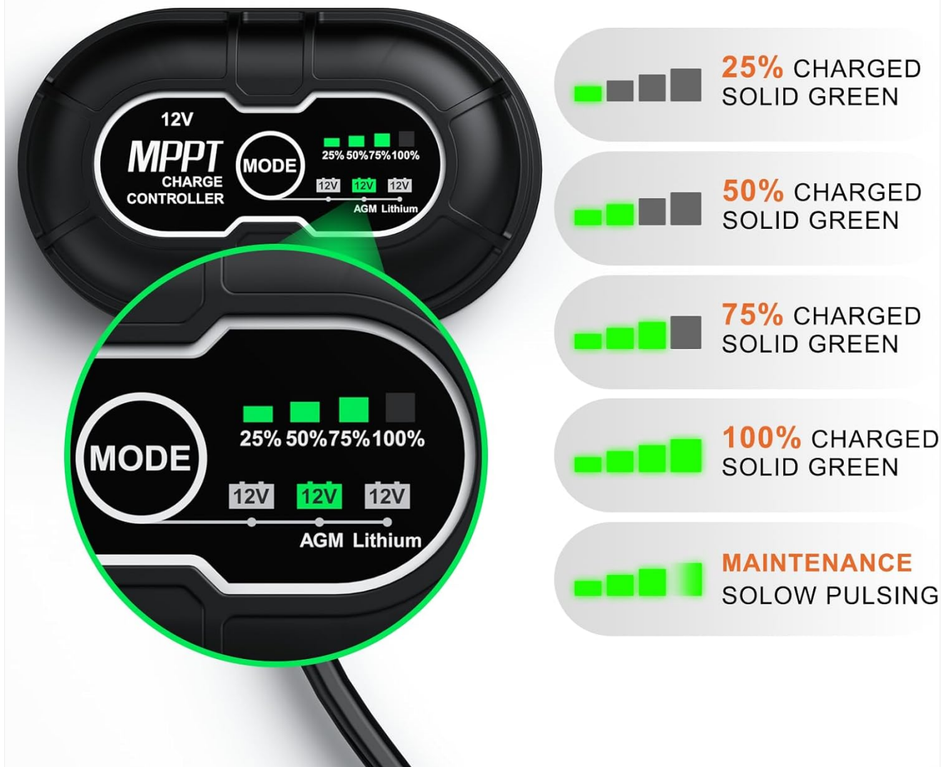
Image 4.2: Interpretation of the charge level LED indicators.
