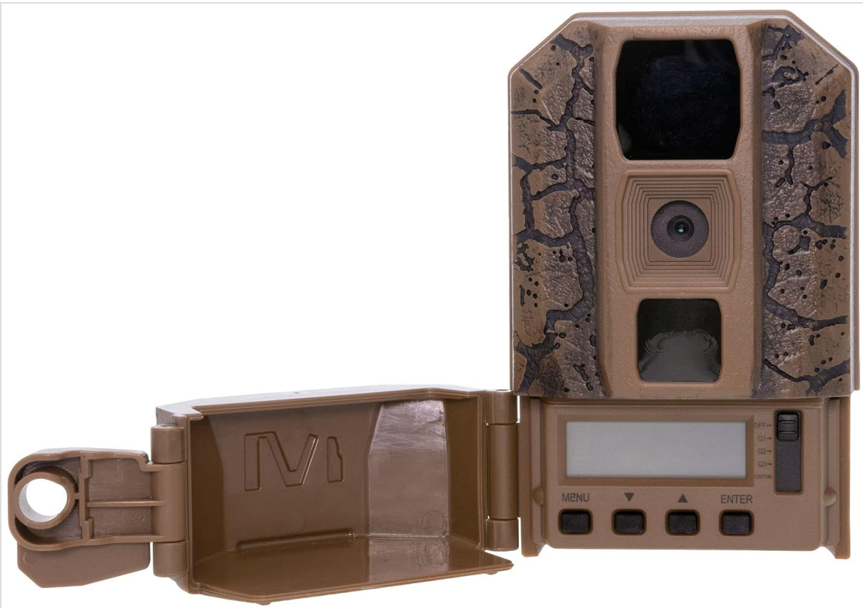
Figure 2: The camera with its front cover open, showing the internal LCD screen, menu navigation buttons (MENU, UP, DOWN, ENTER), and the mode switch (OFF, Q1, Q2, Q3, CUSTOM).
