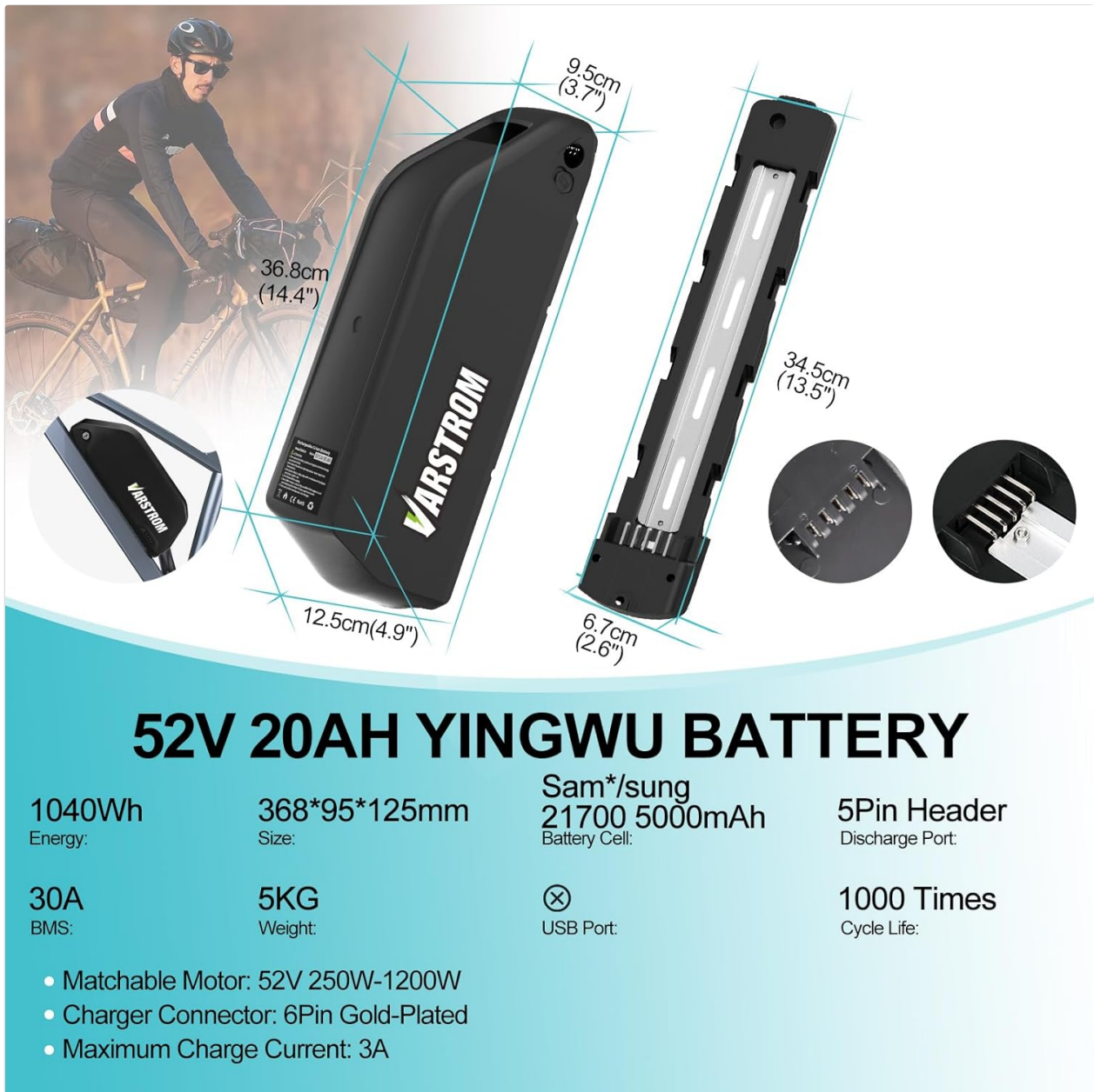
Figure 9.1: This image illustrates the physical dimensions of the battery and highlights key specifications.
