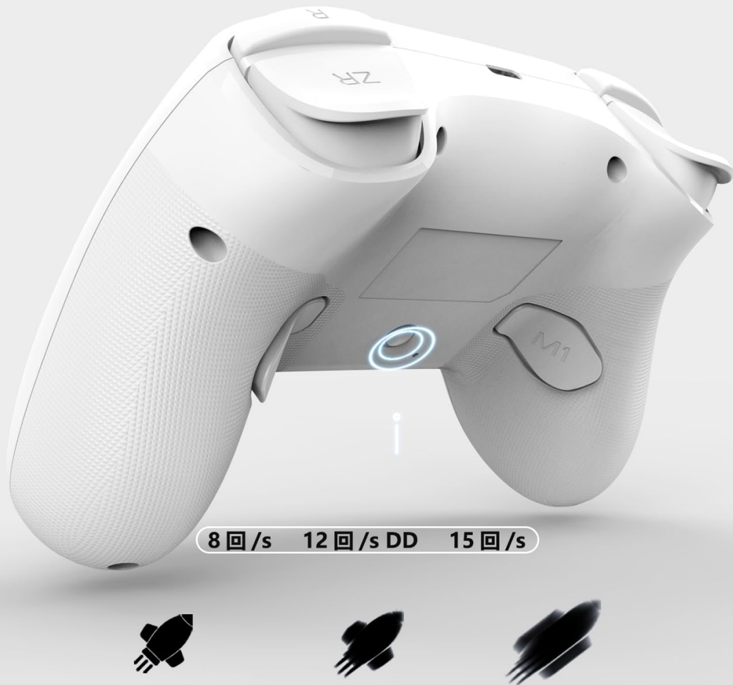
Image: The controller's rear view, demonstrating the TURBO function and its adjustable rapid-fire rates (8, 12, 15 shots/second, note: actual speeds are 5, 12, 20 as per feature bullets).
