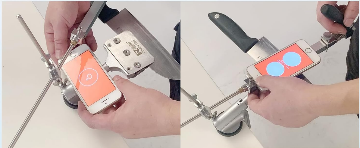
Figure 4: Using a smartphone application to precisely adjust the sharpening angle.
