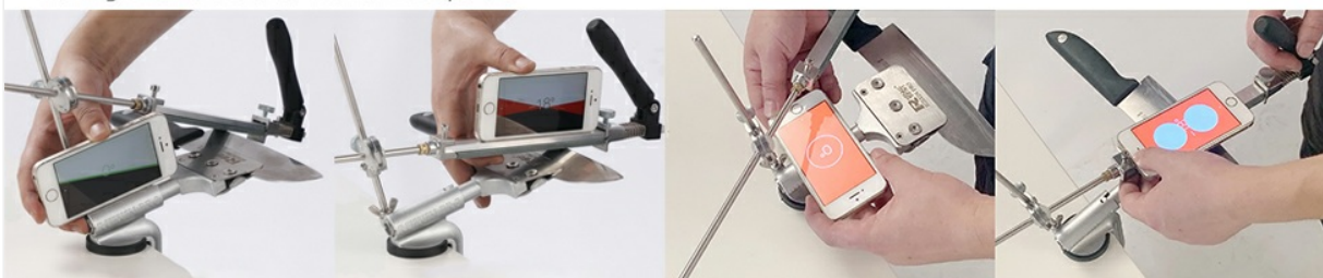
First set the level on the reference surface to zero, then adjust to the angle you need
