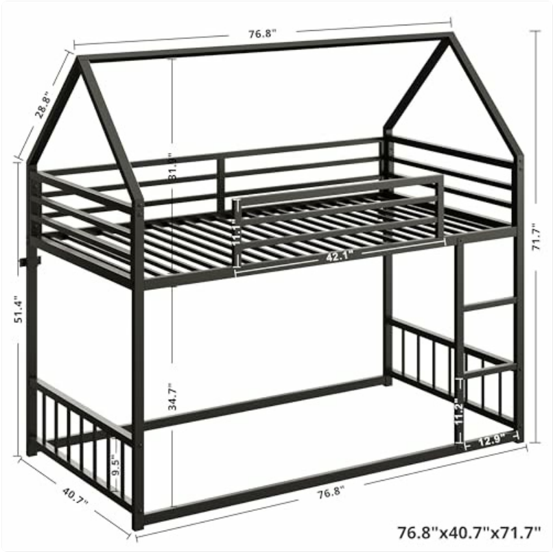
Figure 8.1: Dimensional drawing of the bunk bed.
