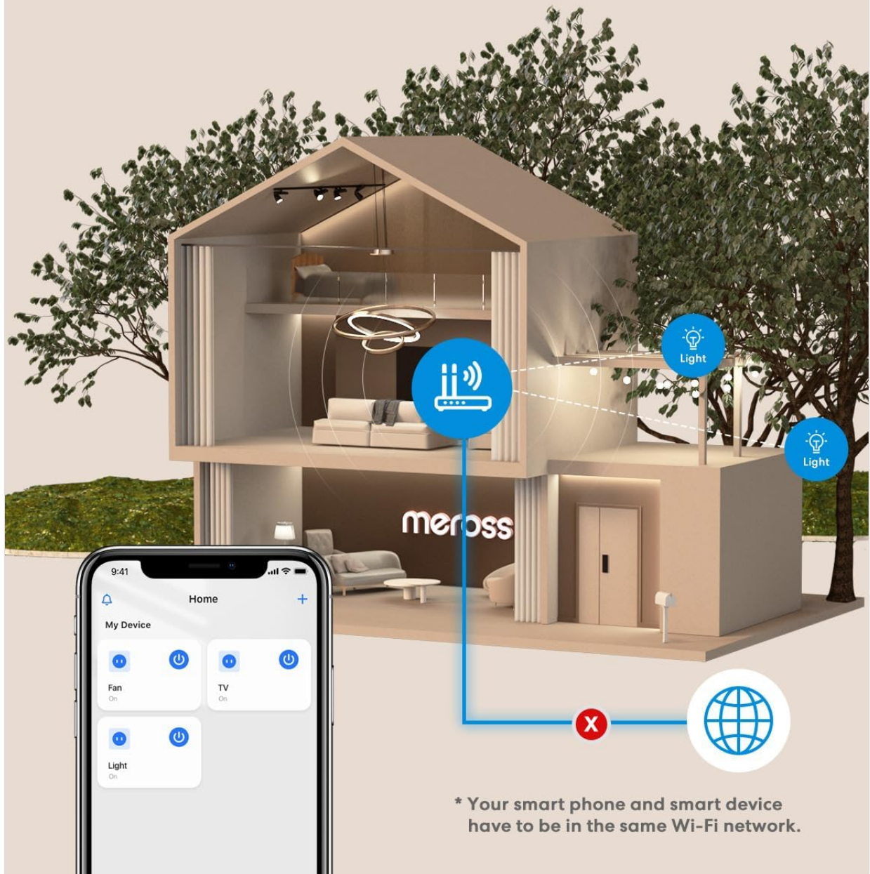
Figure 9: Offline Control. This diagram illustrates how devices can still be controlled via the Meross app within the home Wi-Fi network even if the internet connection is down.
